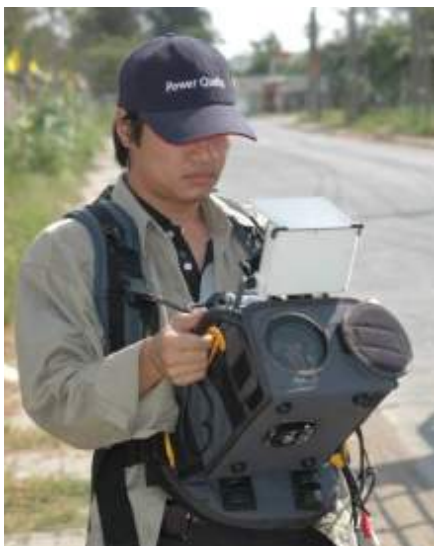
Figure 10: Optical partial discharge detector (left); partial discharge caused by cable touching a tree (right).
